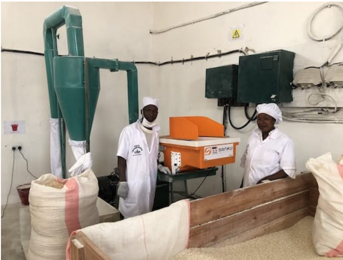
The Sanku dosifier is orange. Bags with pink stripes are sold to millers by PHC-Sanku.
